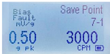
Test Point 2: Known Vibration = 0.50 g pk at 3000 CPM
