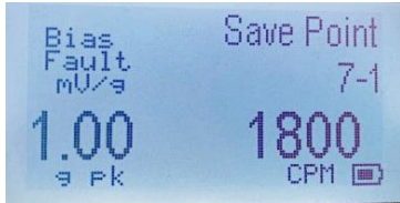
Test Point 3: Known Vibration = 1.00 g pk at 1800 CPM
