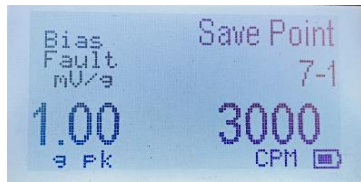
Test Point 4: Known Vibration = 1.00 g pk at 3000 CPM
