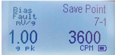
Test Point 5: Known Vibration = 1.00 g pk at 3600 CPM
