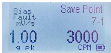
Test Point 4: Known Vibration = 1.00 g pk at 3000 CPM
