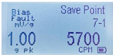
Test Point 6: Known Vibration = 1.00 g pk at 5700 CPM
