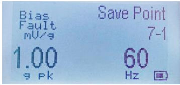
Example known test point in Hz rather than CPM. Not used on sample certificate on next page.
