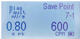
Test Point 1: Known Vibration = 0.80 g pk at 600 CPM
