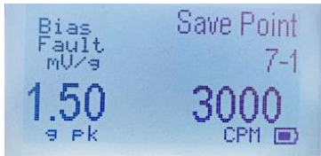
Test Point 6: Known Vibration = 1.50 g pk at 3000 CPM
